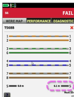
Versiv not only tests the integrity of the shield, but also pinpoints the failure.
